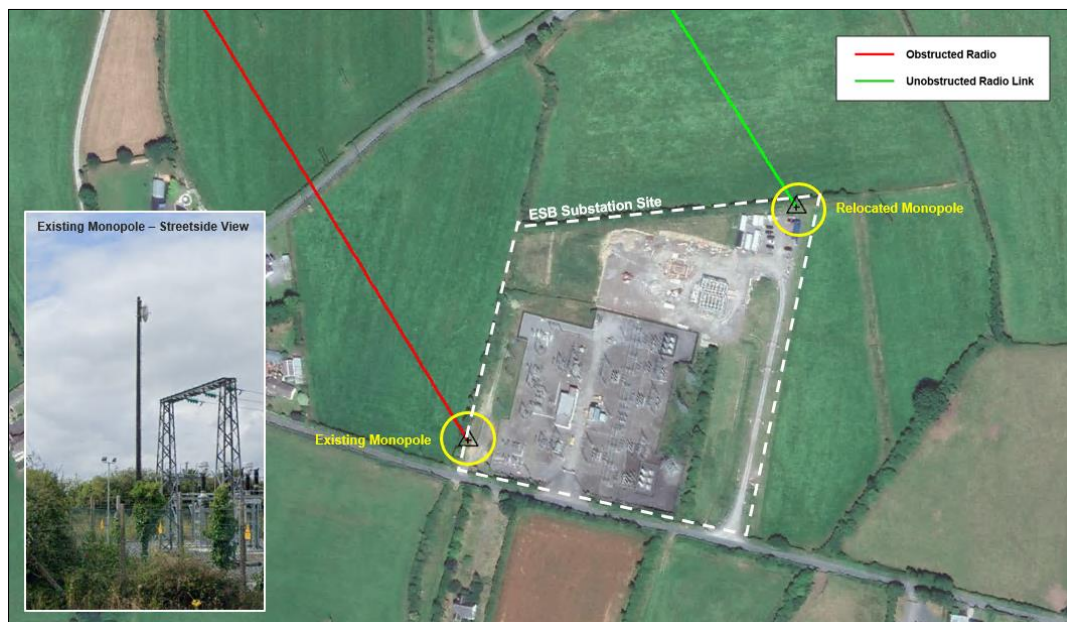
Figure 15. Relocated Monopole – Thurles 110kV Substation
